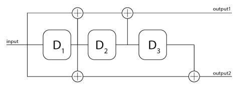
those unfamiliar: There are  $2^3$  states of the coder, one for each possible triplet of most recent bits. The most recent bit is in  $D_1$ , then  $D_2$ , then  $D_3$ . The  $\oplus$  symbol denotes binary XOR. The coder generates (2) output bits, which are then sent over a noisy channel and received on the other end. The added redundancy as well as context-specific output then allows for correcting of some transmittion errors on the receiver side.
